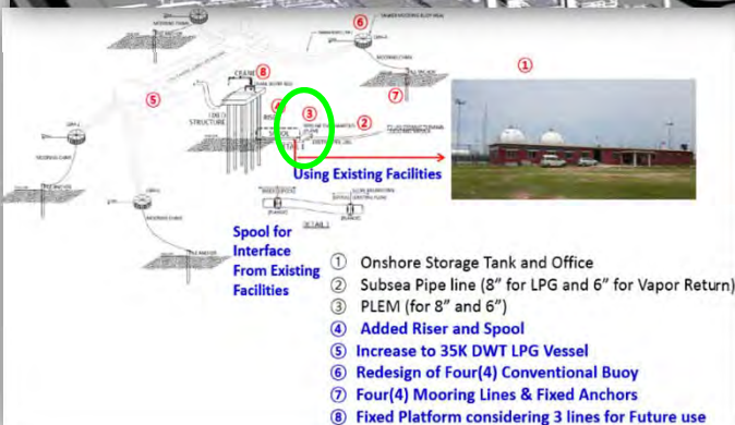
Offshore LPG Terminal Layout(CBM Type)
